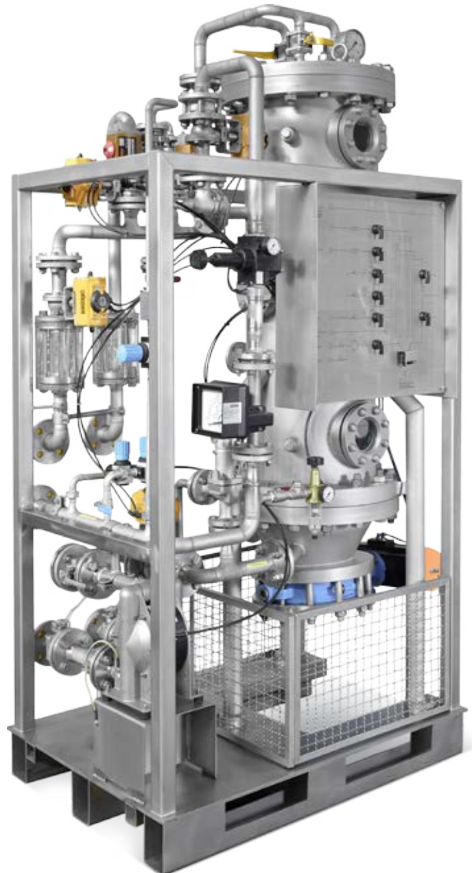
Pilot candle filter plant with 1 m 2 filter area for customer-specific testing on site
