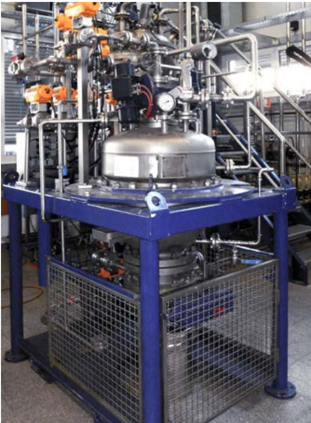
Pilot plate filter skid of type PF 0406 with 0.6 m 2 filter area for customer-specific testing on site
