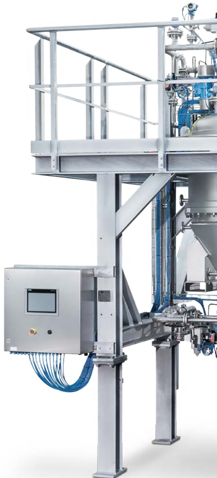
Pressure filter plant of type PF 0713 with 5.8 m 2 filter area
