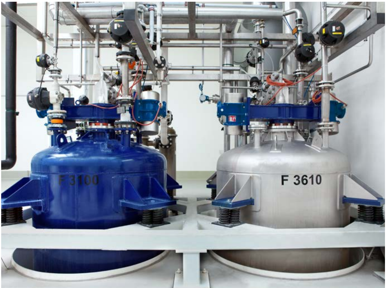
Pressure plate filter of type PF 1018 with 14.1 m 2 filter area (left) and pressure plate filter of type PF 1019 with 14.9 m 2 filter area (right)
