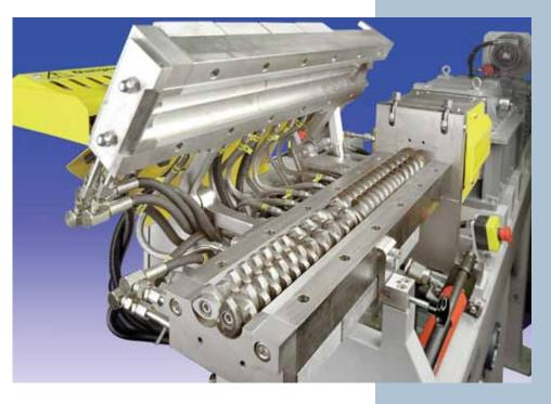
B&P offers a wide range of twin-screw compounding extruders for mixing applications in the plastics industry. For over 60 years, we've been providing mixing solutions to industry that continually advance the state-of-the-art in technology for better finished product quality, higher throughput, and easier operation.
