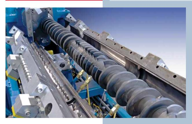
The B&P continuous kneader (CK Series) is a flexible solution for a wide range of compounding needs. This mixer is perfect for a variety of mixing and compounding operations. The system is a single rotating and reciprocating mixing screw which processes material between the moving flights on the screw and the stationary teeth in the barrel wall.
