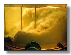
Adding gas to a slurry not only complicates the process requirements of an agitator, it complicates the scaling procedure as well.
