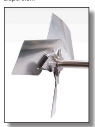
The optimum blade configuration also eliminates the formation of eddy currents on the trailing surface of the blade. This design feature greatly reduces erosion and increases blade life.
