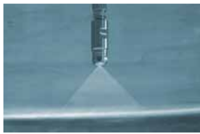
Nozzle atomisation is cost effective low in maintenance and gives maximum control over powder properties.
