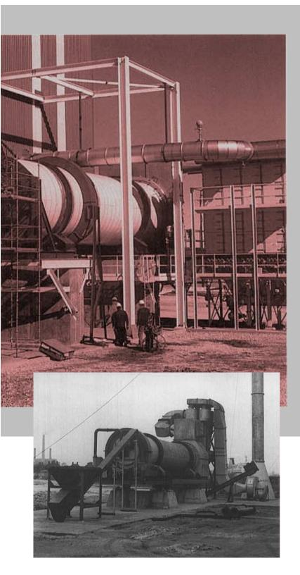
For high temperature processes it is necessary to use either direct fired refractory lined drums or special high alloy steel drums rotating within a refractory lined combustion chaber. Such units operate at temperatures ranging from around 600° C to in excess of 1000°C
