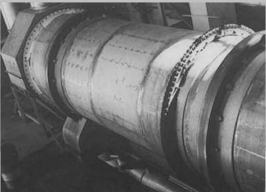
The drying air may be heated directly by means of an oil or gas burner firing into a refractory lined combustion chamber and annulus between the combustion chamber and outer casing. Alternatively, the air may be heated indirectly by means of an air to air, steam to air, thermal oil or electricity heated heat exchanger. Typical drying air temperatures range from 100 C to 700 C.
